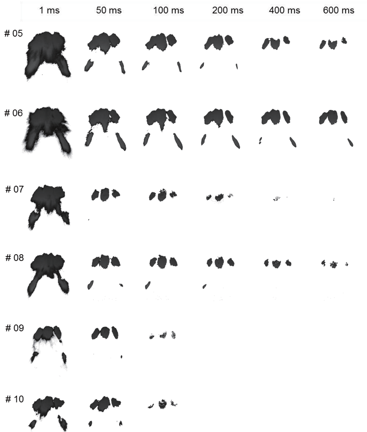
Figure 4.43 Wall wetting images (Case#5~10) after fuel droplet deposit on window surface.
